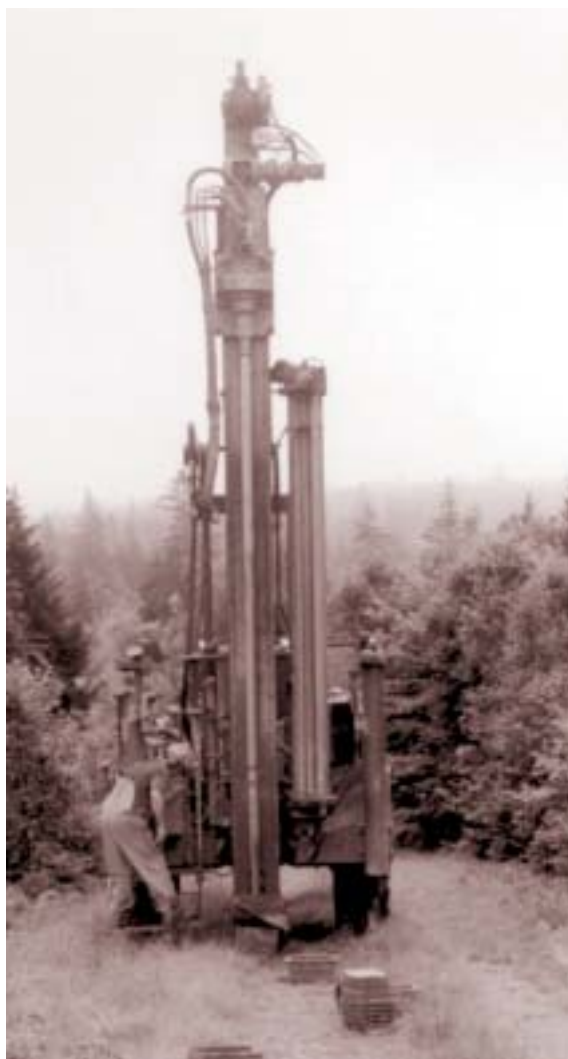
Drill rig operating on the Touquoy reconnaissance percussion drilling program in August 2004
